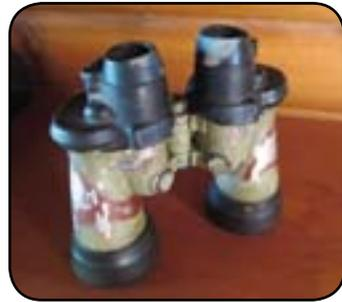
**The binoculars** that inspired this story date from the mid-1900s and belonged to my father. Binoculars allow us to use both eyes when viewing distant objects. They work like two telescopes placed side by side providing a three dimensional image. The area seen through binoculars is called the field of view.
